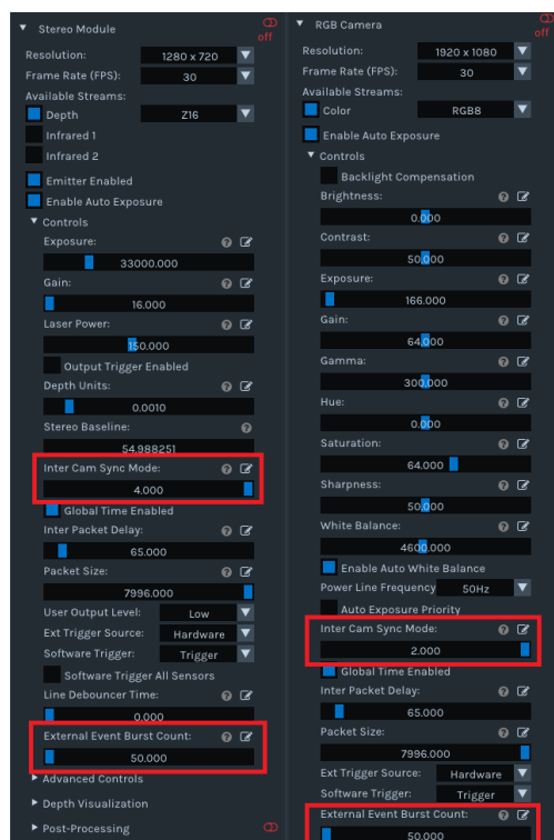
Figure 15 – Setting camera operating mode to external event burst mode for Rolling Shutter cameras
