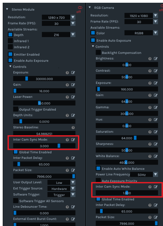
Figure 14 – Setting camera operating mode to external event mode for Rolling Shutter cameras
