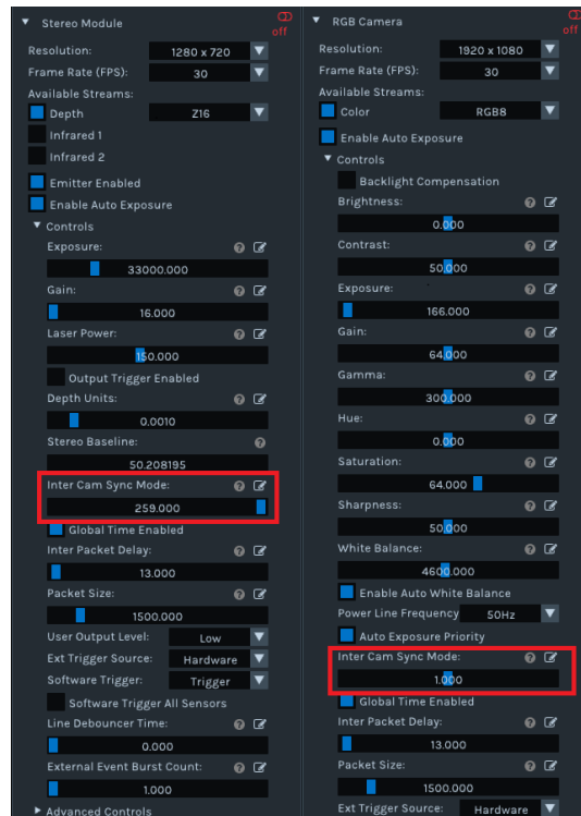
Figure 12 – Setting camera operating mode to external event mode for Global Shutter cameras
