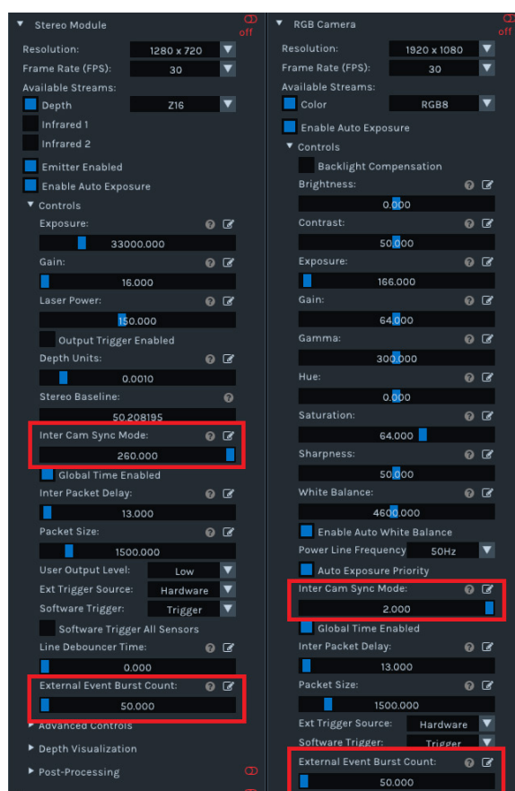
Figure 13 – Setting camera operating mode to external event burst mode for Global Shutter cameras
