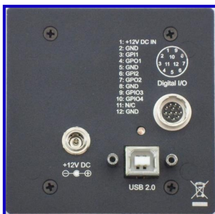
Figure 31: Lm11059 header and pin numbering.
