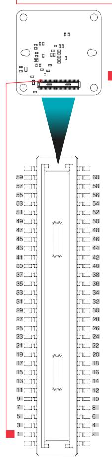
Note Signals are routed directly from image sensor to connector. Details on specific signals are described in the respective Sony® image sensor datasheet.
