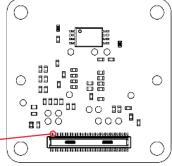
**Note** Signals are routed directly from image sensor to connector. Details on specific signals are described in the respective Sony® image sensor datasheet.
