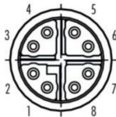
Figure 1 – M12 Connector PIN Layout
