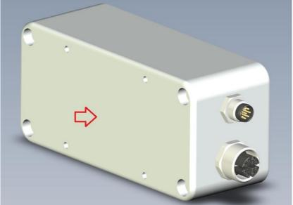
Figure 3 - Hottest Part of the Camera Housing
